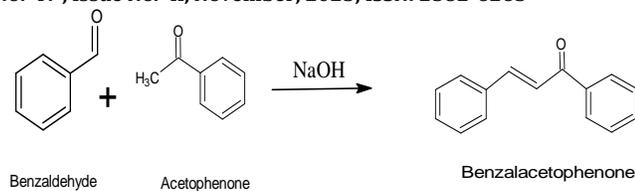
**Aldol Condensation:** Benzaldehyde and acetophenone reacts and lose water molecule by heat give chalcones [15].
