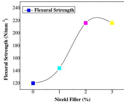
**Fig. 2 Effect of flexural strength on nickel powder filled 6061 aluminum alloy composites**
