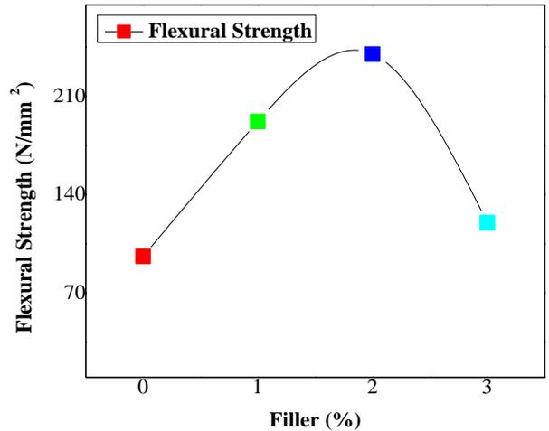
**Fig.4 Effect of flexural strength on nickel powder filled 6061 aluminum alloy composites**
