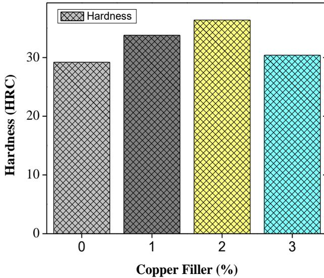
**Fig.3 Effect of Hardness on Copper Metal Powder Filled Al 6061 Alloy Composites**
