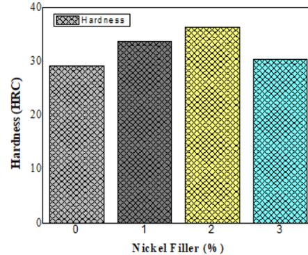
**Fig. 1 Effect of Hardness on Nickel Metal Powder Filled Al 6061 Alloy Composites**
