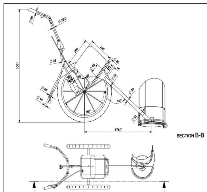
**Fig 1: 2-D View of harvester with 35.8cc Engine**
