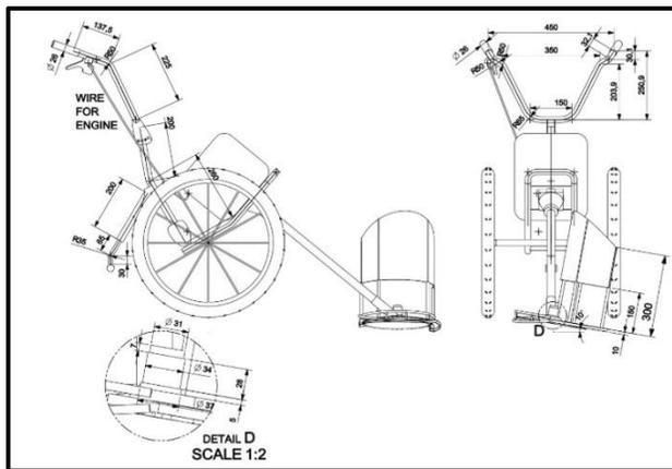
**Fig 5: 2-D View of harvester with 35.8cc Engine**
