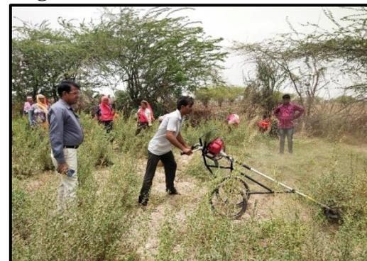
(ii) A more powerful engine of 47.9 cc was thus selected to overcome difficulties incurred in undulated fields. Field test with the engine revealed its suitability under undulated field conditions (Fig 7).
