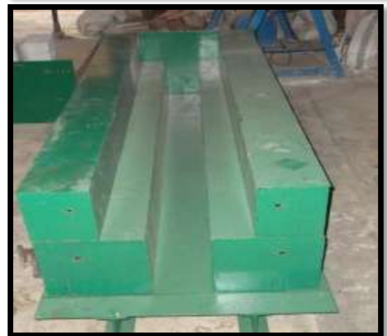
Fig. 2: Moulds for casting of T-beam
